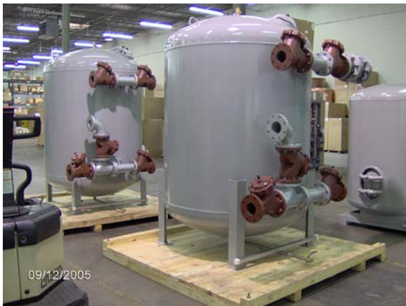
Pre – Treatment pressurized filters
