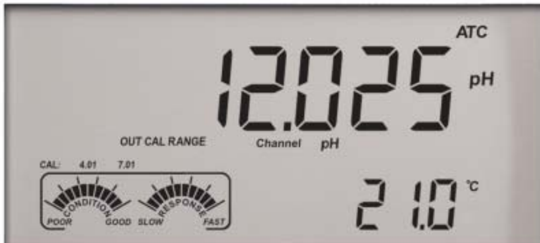
pH channel on display with out of calibration range warning - LCD shown actual size
